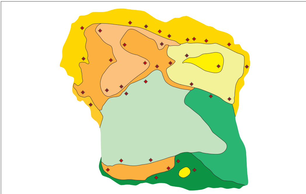
Figure 4 → Example of an SHM Map. All zones are “susceptible to amplification” (soft soils above geological bedrock). The red dots represent the location of investigations that allowed for the identification of different zones (the symbol indicates a generic investigation and has no reference to the symbology used in the Graphic and Data Archiving Standards). The 3 conditions described in Chapter 2.1 have not yet been analysed at this stage.
