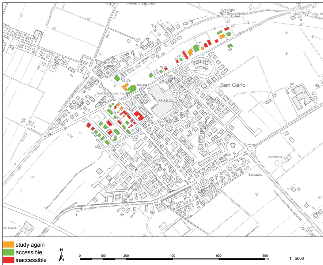
Figure A3.2 → Building damage classes in areas with geotechnical problems.
