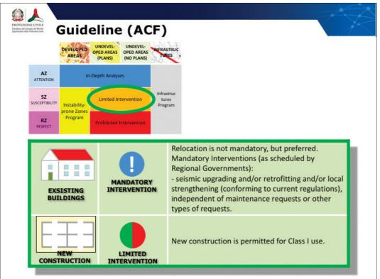
Slide  $4 \rightarrow$  Susceptibility Zones for Undeveloped Areas (with or without plans for development): Mandatory interventions for existing buildings and Limited Interventions for new construction.
