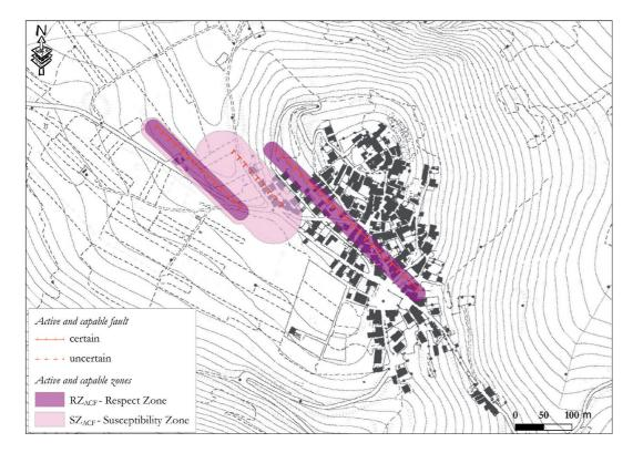
Drawing 1  $\rightarrow$  Susceptibility Zone (SZ<sub>ACF</sub>) and Respect Zone (RZ<sub>ACF</sub>) for active and capable faults on a Seismic Microzonation Map (Level 3 SM).
