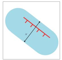
fusion of all polygons to obtain an asymmetrical polygon with respect to the segment of the fault, equal to the dimensions (x) of the zone.
