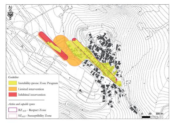
Drawing  $3\to$  Guidelines for Susceptibility Zones (SZ<sub>ACF</sub>) and Respect Zones (RZ<sub>ACF</sub>) of ACF (minimum perimeter).
