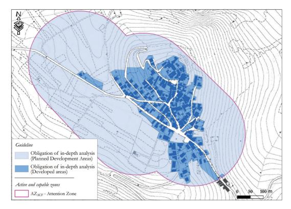
Drawing 3  $\rightarrow$  Guidelines for Attention Zones (AZ<sub>ACF</sub>) of active and capable faults.
