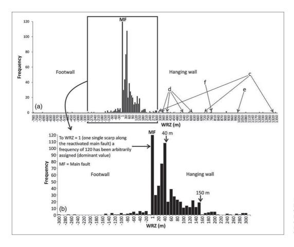
Figure A3.1  $\rightarrow$  Statistics on the frequency of breakage as a function of the distance from the main fault plane (Boncio et al., 2012). WRZ (width of the rupture zone) indicates the width of the zone affected by coseismic ruptures, measured perpendicular to the direction of the main fault (Main Fault, MF).
