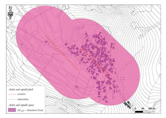
Drawing 1  $\rightarrow$  Attention Zone (AZ<sub>ACF</sub>) of active and capable faults on a map of Seismically Homogenous Microzones (Level 1).
