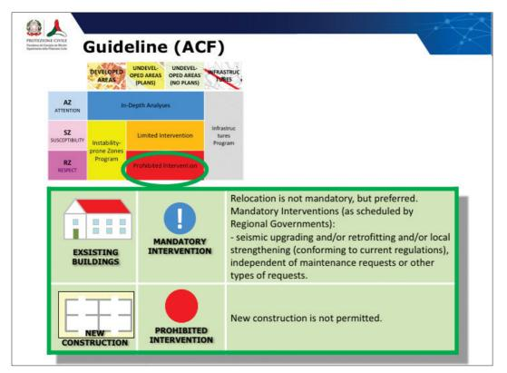
Slide  $5 \rightarrow$  Respect Zones for Undeveloped Areas (with or without plans for development): Mandatory interventions for existing buildings and prohibition of any new construction.
