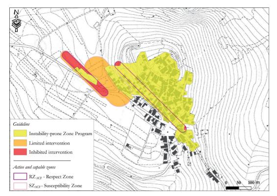
Drawing 4  $\Rightarrow$  Guidelines for Susceptibility Zones (SZ<sub>ACF</sub>) and Respect Zones (RZ<sub>ACF</sub>) of active and capable faults (maximum perimeter).
