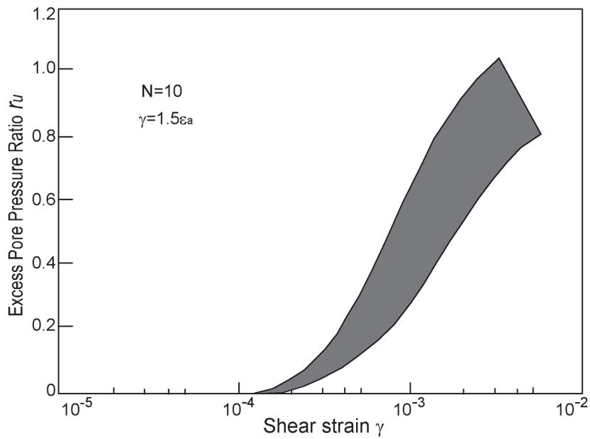
Figure 2.7-3 – Pore pressure ratio  $r_u$  vs. maximum shear deformation induced by the earthquake
