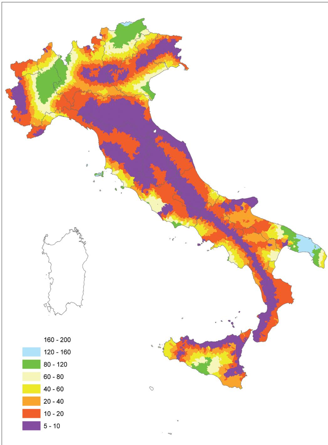
Figure 2.8-5 – Modal values of R for each Municipality, obtained by disaggregating the hazard with return periods of 475 years (processing of data from Spallarossa & Barani, 2007).
