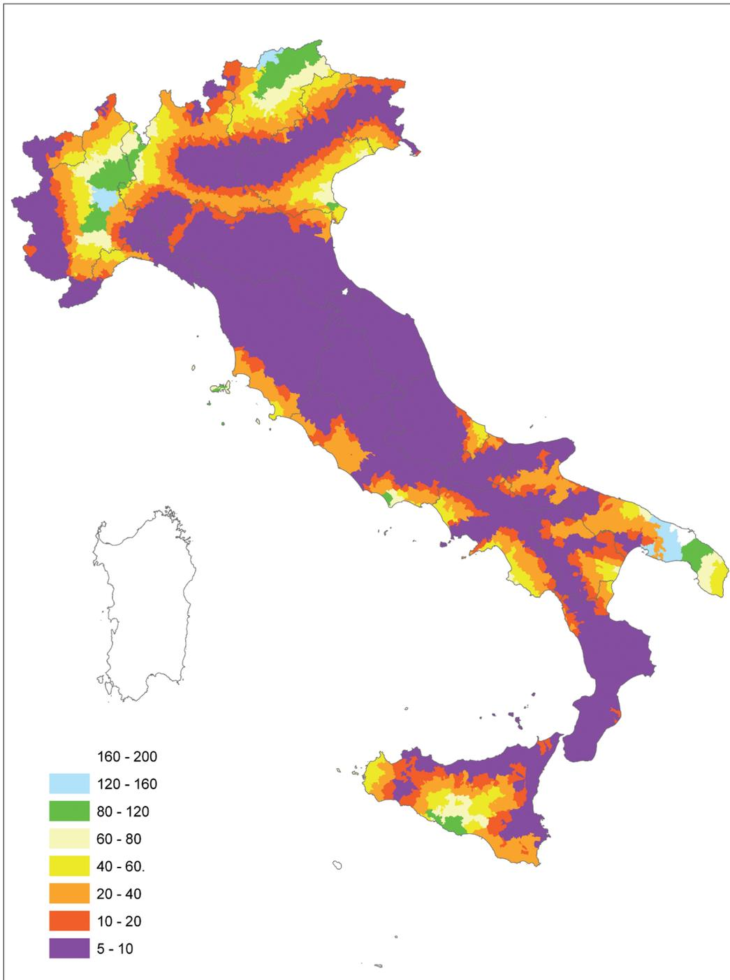
Figure 2.8-4 – Modal values of R for each Municipality, obtained by disaggregating the hazard with return periods of 475 years (processing of data from Spallarossa & Barani, 2007).
