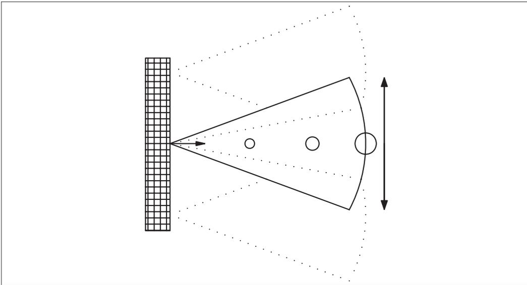
Figure 2.6-3 – Plan view of a shadow cone containing the most likely run-out trajectory
