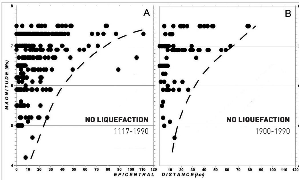
Figure 2.8-6 – Observed liquefaction phenomena in terms of  $M_s$  and epicentral distance (from Galli, 2000)
