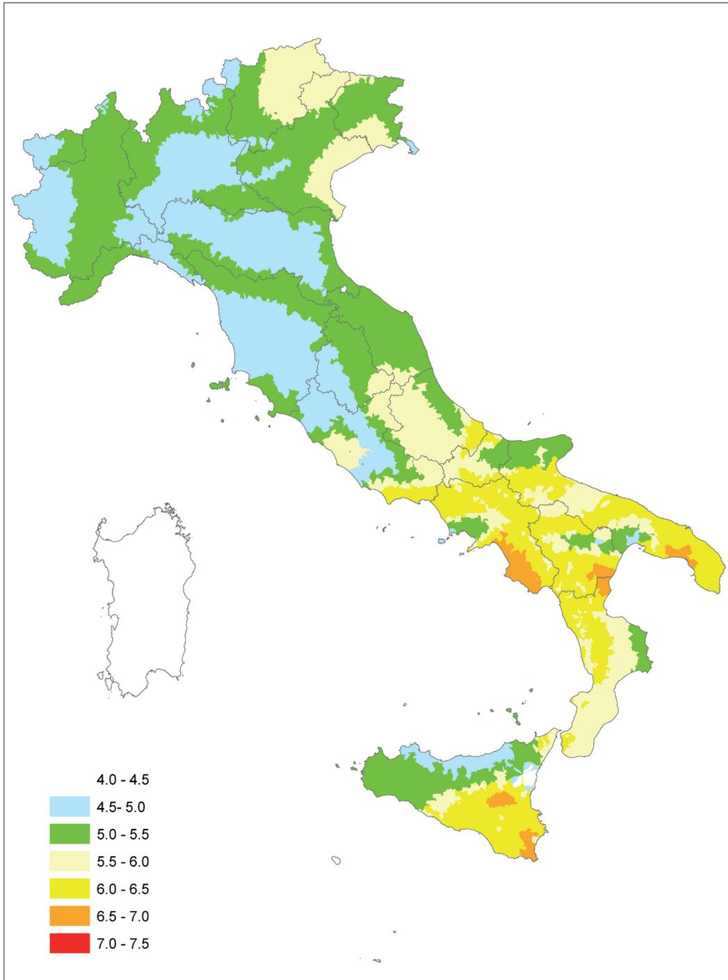
Figure 2.8-3 – Modal values of M for each Municipality, obtained by disaggregating the hazard with return periods of 475 years (processing of data from Spallarossa & Barani, 2007).
