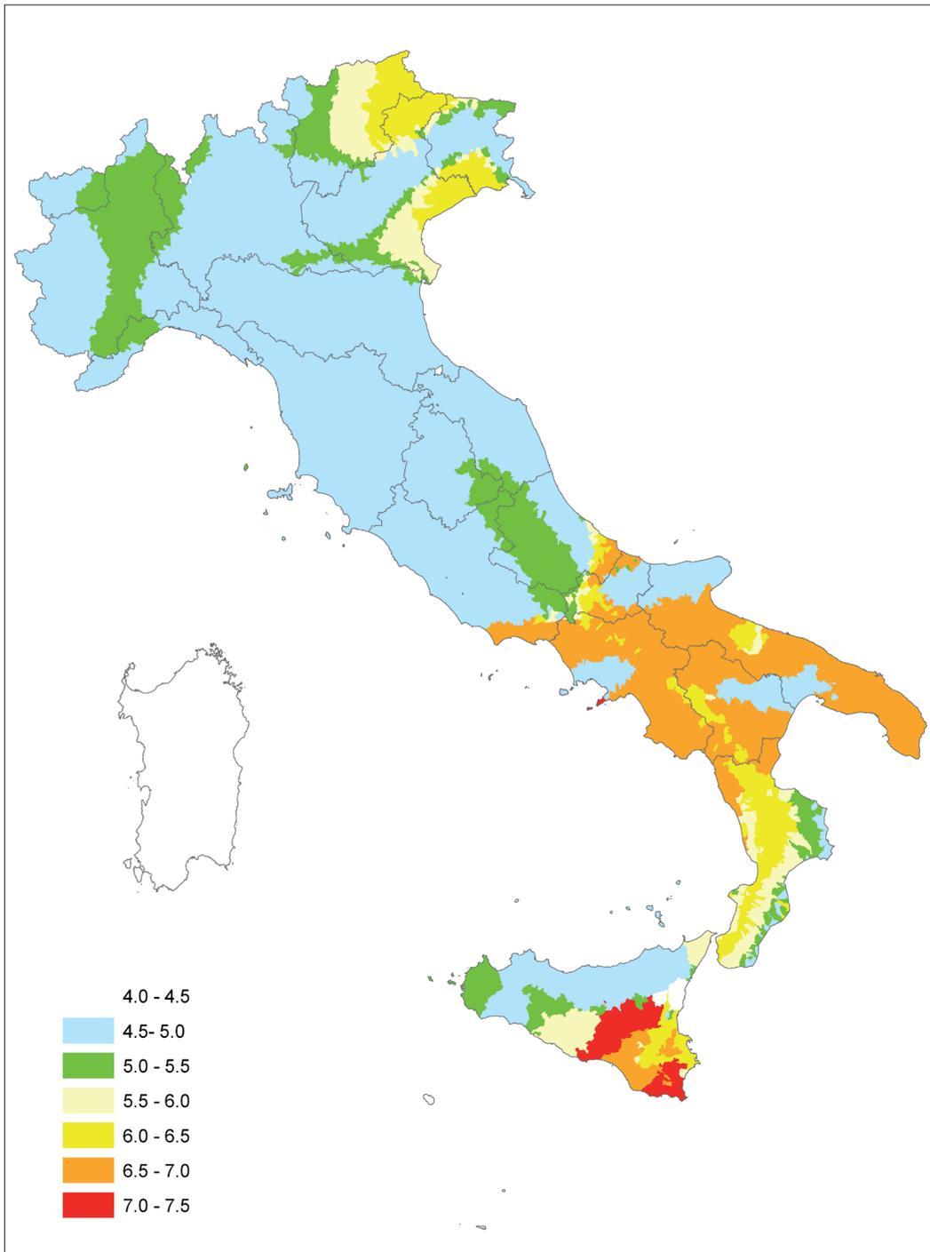
Figure 2.8-2 – Modal values of M for each Municipality, obtained by disaggregating the hazard with return periods of 475 years (processing of data from Spallarossa & Barani, 2007).
