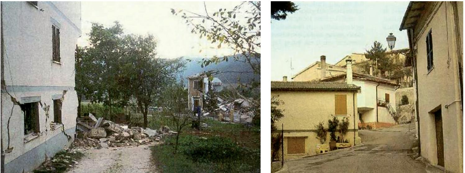
Figure 1.1- 2 – Umbria-Marche earthquake, 1997. Differences in damage to neighbouring sites due to local effects. Left, Cesi Bassa (IX MCS); right, Cesi Villa (VII MCS).
