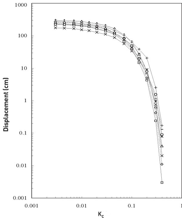
Figure 2.6-1 – Induced permanent displacement – critical seismic coefficient for 8 artificial, spectrum-compatible accelerograms on stiff soil A, seismic zone 2, for an indefinite slope (Cavalera & Brancucci, 1995)
