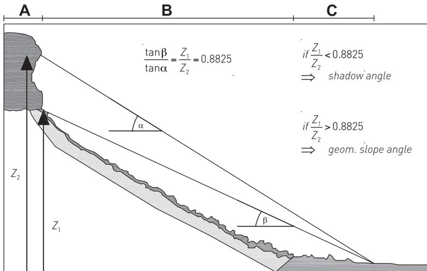
Figure 2.6-2 – Soil parameters for applying the method proposed by Onofri & Candian (1979)
