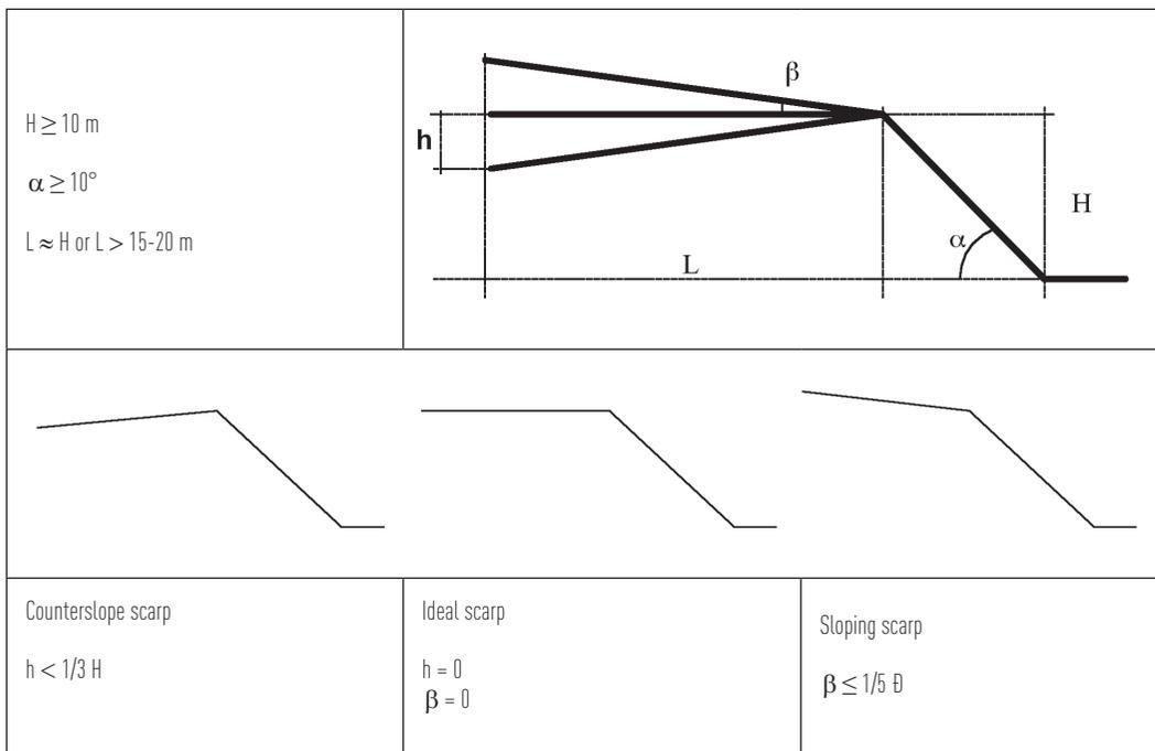
Figure 2.5-2 – Reference diagram for the scarp and identification criteria.
