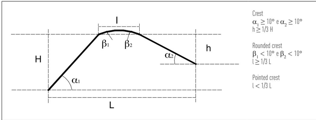
Figure 2.5-1 – Reference diagram for the crest and identification criteria.
