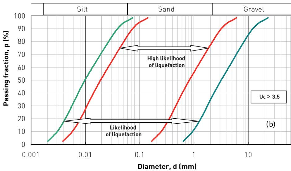
Figure 2.7-1 – Grain sizes for preliminary assessment of the liquefaction susceptibility of a soil (soils of uniform grain size (a) and extended grain size (b)) (from AGI, 2005).
